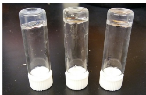
Figure 1. Gels of 6 wt % 40PVAc/0.3 wt % BDBA in methanol, DMSO, and THF (left to right) 7 days after preparation.
